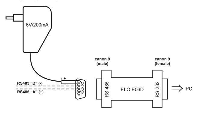
The ELO E06D converter is an optional accessory for connection of transmitter/transmitters with RS485 interface to the PC via serial port RS232. Connect connector marked RS232 directly to the PC, connect power to connector marked RS485. Power voltage +6V DC from an external acdc adapter connect to pin 9, 0V connect to pin 5. Also mutually connect pin 2 and pin 7. Link RS485 is connected across pin 3 (A+) and pin 4 (B-).
