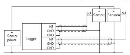
Legend of connection of connector ELKA: INx – brown (input) GND – blue (ground) GND – black (shielding)
